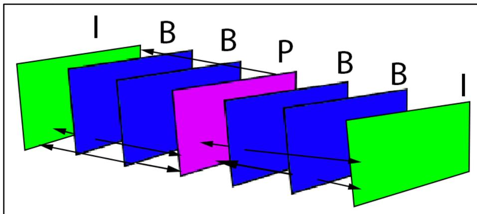
Figure 6. Illustration of the relationship between I-frames, P-frames, and B-frames
